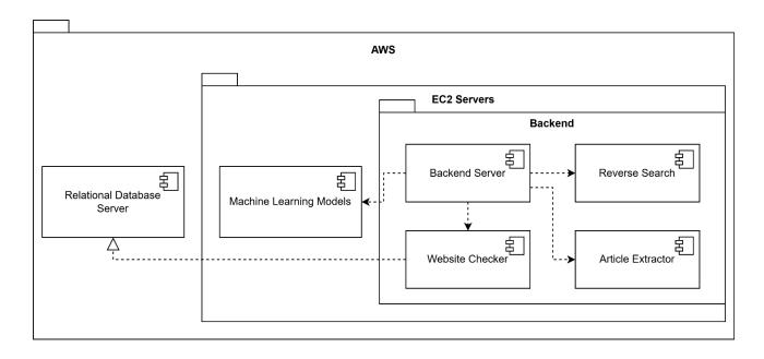
The AWS Subsystem forms the core backend infrastructure, responsible for handling fact-checking requests, processing machine learning models, managing data, and ensuring system reliability. The backend is designed to efficiently process high volumes of requests while maintaining security and scalability.
