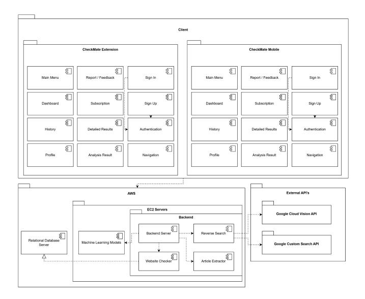
CheckMate consists of four main layers: Client Layer, AWS Layer, External APIs Layer, and Backend Logic Layer.
